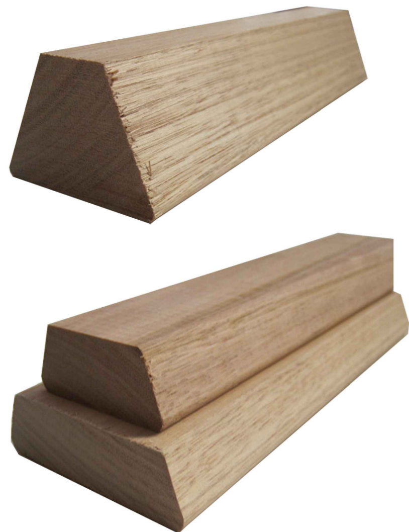
(Left Top) - Silvertop Ash (Eucalyptus Sieberi) Bevelled Edge Board Seasoned (KD) DAR- 55x40mm, (Rated bushfire resisting timber to maximum BAL 29 as per AS 3959 ), Termite resistant ( AS 5604 ) and natural durability rated as Class 2 above ground up to 25 years)
