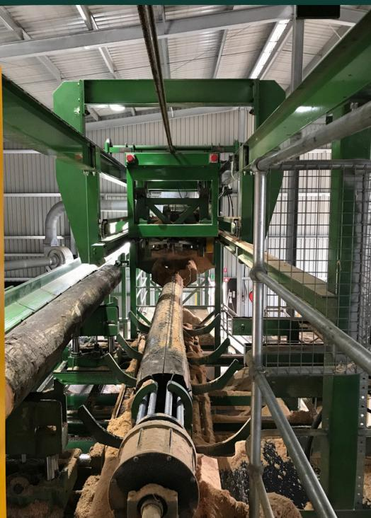
Radial Sawing was specifically designed to maximise the recovery of sawn timber from smaller logs. As such, Radial Sawing has a range of both environmental and technical benefits. Where conventional sawing methods require large diameter logs. Radial Sawing technology helps make native hardwood plantation logs more viable by maximising the yield of high value timber products from much smaller logs.
