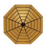
Radial sawing works by quarter sawing a log into wedges (like a pizza) from these wedges the log is then back sawn into varying sizes of bevelled edge boards. These bevelled edged, rough sawn boards can be used unseasoned (green) for products such as Board & Batten or Screening. Alternatively the boards can be racked out for air drying, to then be kiln dried and moulded into high quality profiles such as Shiplap Cladding or Decking.
