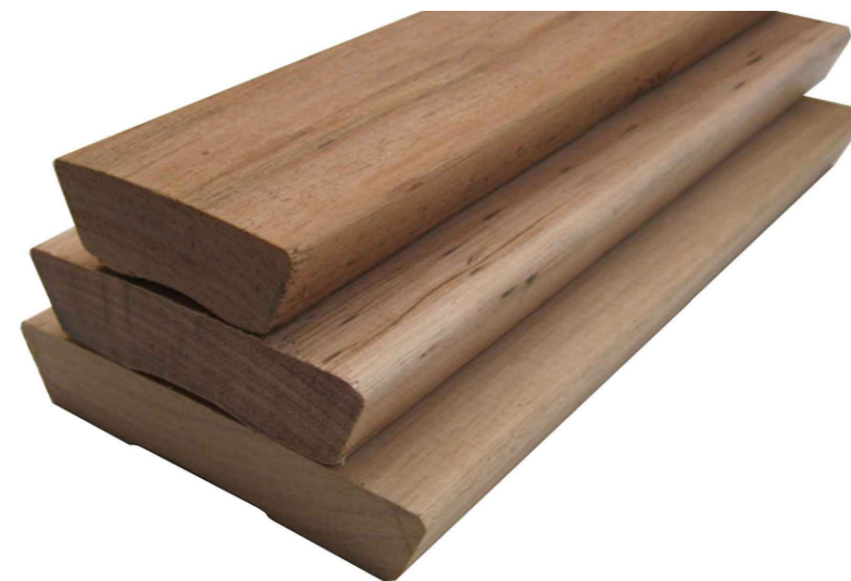
(Left) Yellow Stringybark (Eucalyptus Muelleriana) - 55x19 & 80x19 & 100x19mm (Suitable for areas rated BAL19 or less for bushfire resisting timber as per AS 3959 ), Termite resistant ( AS 5604 ) and natural durability rated as Class 2 above ground up to 25 years)
