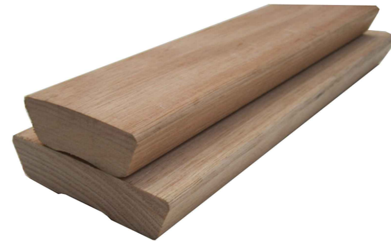
(Left) Silvertop Ash (Eucalyptus Sieberi) New Deck Profile - 55x19 & 80x19mm (Rated bushfire resisting timber to maximum BAL 29 as per AS 3959 ), Termite resistant ( AS 5604 ) and natural durability rated as Class 2 above ground up to 25 years)
